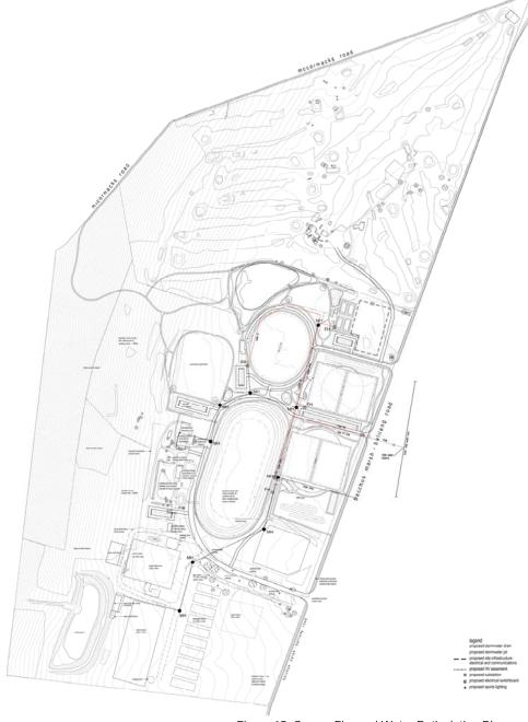
Figure 15: Sewer, Fire and Water Reticulation Plan
