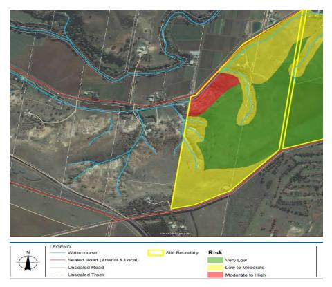
Figure 4 – Sodic Soils within the Stonehill Development
