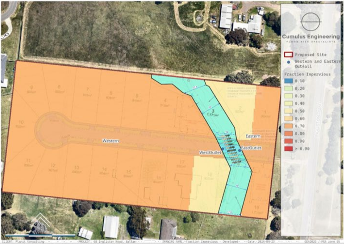
FIGURE 2-4 POST DEVELOPED VALUES OF FI
