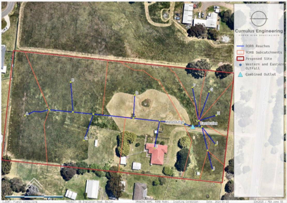
FIGURE 2-2 RORB MODEL SCHEMATISATION UNDER EXISTING CONDITIONS
