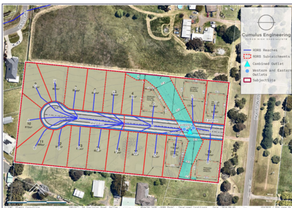
Figure 7-1 Developed Conditions Catchment Delineation
