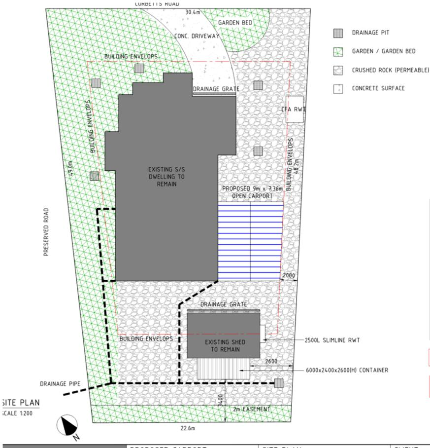
AREA ANALYSIS 275 SQ.M EX. HOUSE EX. SHED 60 SQ.M CONC. DRIVEWAY 50 SQ.M PROPOSED CARPORT 66 SQ.M SITE AREA 1230 SQ.M SITE COVERAGE 385 (31.3%) PERMEABLE AREA 845 (69%)
