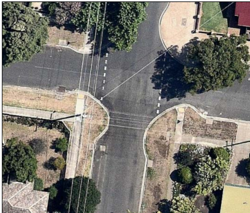
Figure 4-7 Road Narrowing Treatment (Graham St / Pilmer St, Bacchus Marsh)
