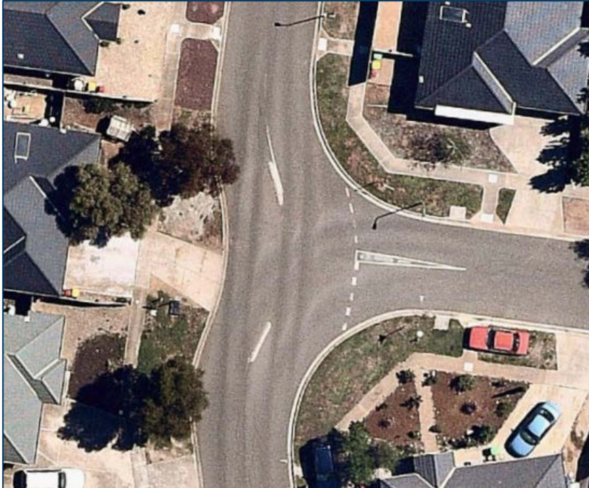
Figure 4-3 Modified T Intersection (Burbidge Dr / Lone Pine Sq, Bacchus Marsh)
