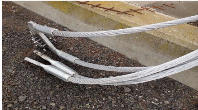
Figure 7: Four bundled conductors
