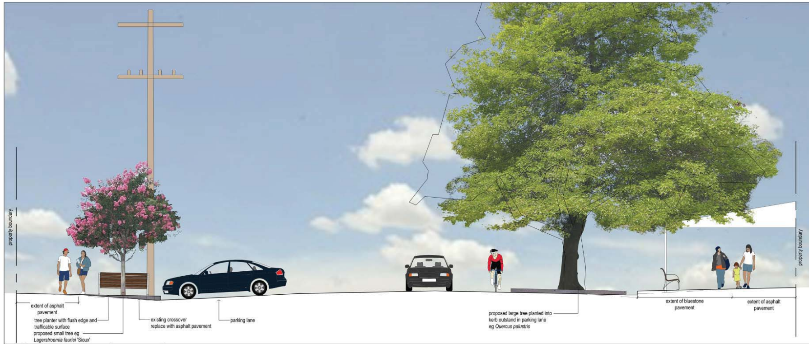
section CC typical road cross section
