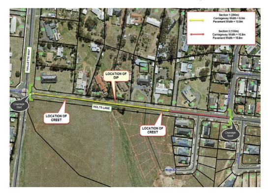
The road is within a 'General Residential Zone' (GRZ) area and the southern side of Holts Lane is abutting the new Clifton Park North subdivision. The road section between Cunningham Close and No. 102 Holts Lane has 8.0m surface width and kerb and channel on south side of Holts Lane.
