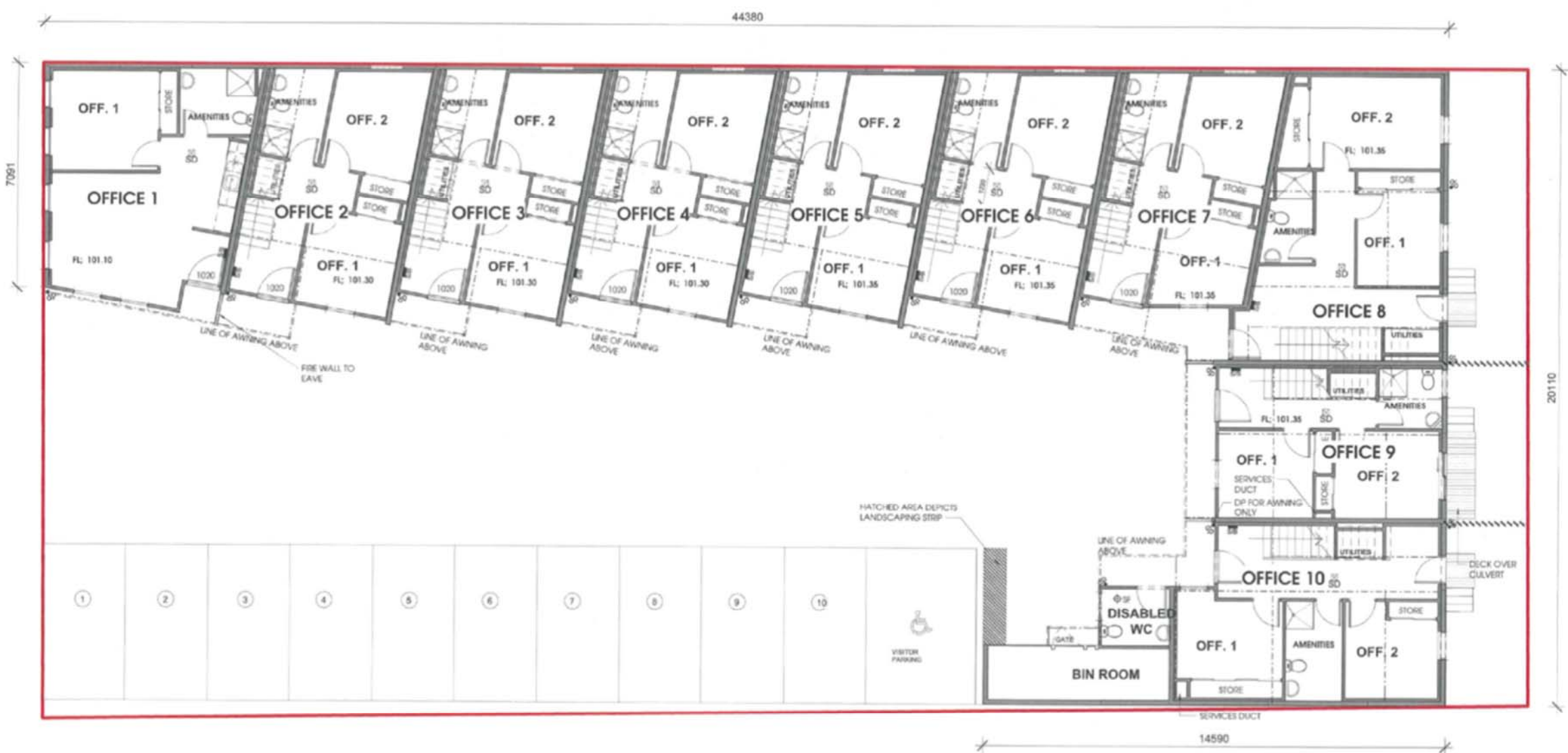
EXISTING CONDITIONS GROUND FLOOR PLAN SCALE 1:100
