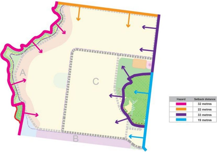
Figure 1: Areas A, B and C, hazard interfaces and relevant bushfire setbacks
