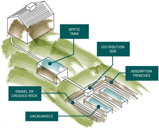
The surface of this trench area needs to be kept free of structures (e.g. sheds), paving, deep rooted trees etc, to ensure the trenches continue to work efficiently.
